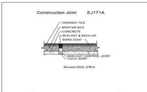
Now let's take a look at a contraction/control joint. Again, the term "control" refers to a type of movement joint which is cut or sawed into the body of a slab which creates a weak point where a crack would then be most likely to occur. Normal depth of the saw cut is 1/2" to 3/4" of an inch. It is important to note that a control joint must be sawed into the slab while the concrete is still "green", that is, while it is still in the curing process.
