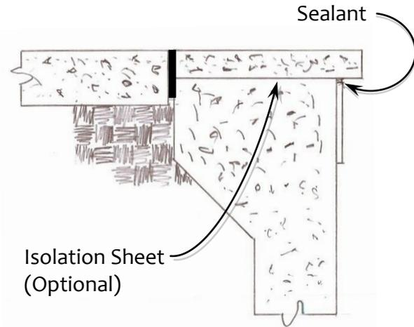
3) Pre-Cast Coping: This coping is generally cast into molds off-site using concrete or pressed clay, allowed to cure and then brought to the site for installation. It's made in straight pieces, end caps, and varying radius's that will accommodate different pool shapes.
